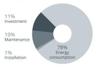
Over a 5-year lifetime, the total cost of compressed air production includes 78% energy costs if a standard compressor is used.
