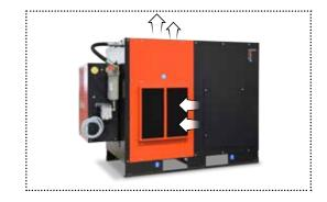
Cooling is an important factor during the compressed air production process, as it helps to increase system efficiency and reliability. **The new Blade 8-12 i is equipped with an electric fan with an integrated inverter.** The rotation speed of the cooling fan adapts itself to the working conditions and the environment, optimizing performance and allowing safe operation up to an ambient temperature of + 46 ° C.
