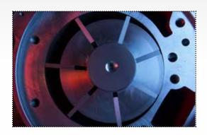
Mattei airends rotate slower than other types of compressors and their blades slide frictionless on a thin film of oil which ensures complete reliability. Mattei machines also have fewer moving parts than other compressors and as the rotor runs on bushes, it has a **virtually unlimited lifespan**.
