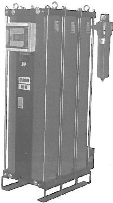
X-DRY 300-1050 modular adsorption dryers are designed for continuous separation of water vapour from compressed air thus reducing dew point. Operation of dryer requires two columns operated alternately. Adsorption takes place under pressure in first column while second column regenerates with a portion of already dried compressed air at ambient pressure.
