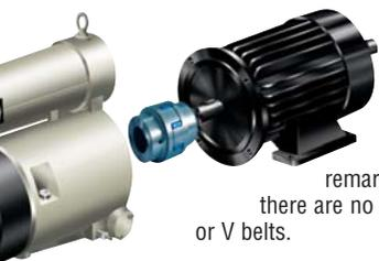
The electric motor and the compressor are coupled directly by means of flexible coupling and turn at only 1500 rpm.
