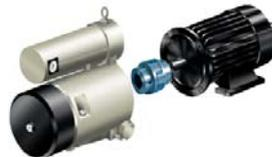
The electric motor and the compressor are coupled directly by means of flexible coupling and turn at only 1500 rpm. Direct coupling determines a remarkable "energy saving" because there are no energy losses caused by gears or V belts.
